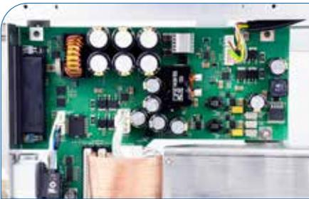
› The power electronics is now integrated in the print mechanics. Thus, it was possible to use only one cable
