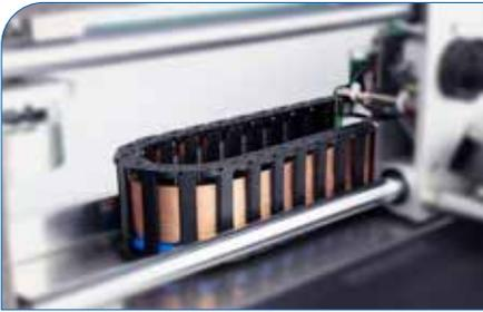
› Only one energy chain left. This can be opened on the inside. The inside separators prevent the flat ribbon cables from touching the pneumatic hose.
