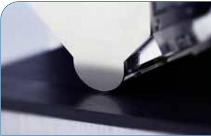
› By a folded edge, the transfer ribbon is guided around the printhead edge. This facilitates inserting the ribbon
