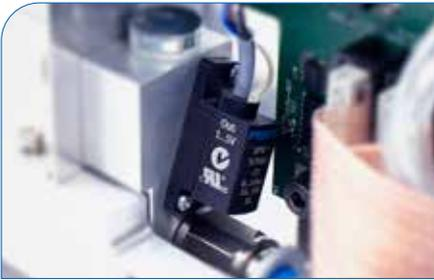
Connection block with piezoresistive pressure sensor with analogue output voltage for 'intelligent' monitoring of the compressed air supply.
