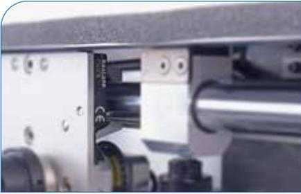
To detect the end positions, inductive sensors are now used. They are less soil-sensitive.
