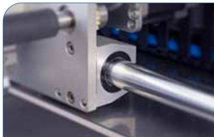
Hard chromed guiding shafts with ball bushings provide a very stable linear guiding. They are easy to adjust and align - even on site at the customer.
