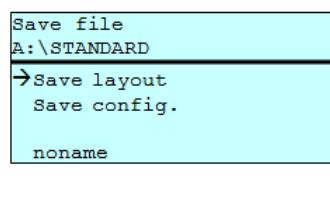
If an USB keyboard is attached a new file name for *noname* can be assigned.
