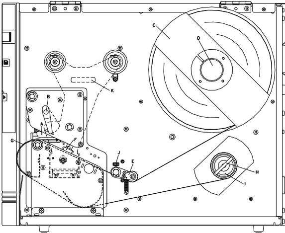
In rewind mode the labels are wound up internally after printing for later use.
