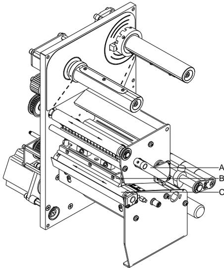
A soiled pressure roller can lead to a reduced print quality and can affect the transport of material.
