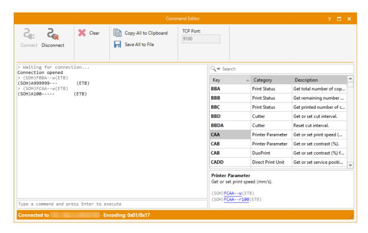
Enter a CVPL command in the command line, or select a command from the list and click on the related link. Press **[ENTER]** key to execute the command. A complete description of the supported CVPL commands can be found in the interface description of your Valentin printer.
