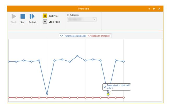
Click **Test Print**, or **Label Feed**, or slowly pull the label. If the photocell is configured correctly, the value drops as soon as the photocell detects the gap between the labels.
