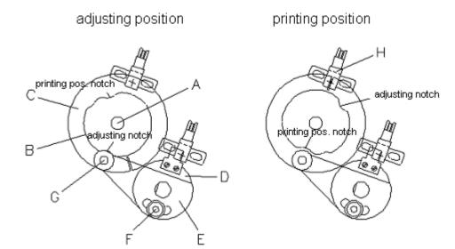
The illustration shows the axe of the ribbon savings motor (A) with pressure curve (B) and disc (C) from the rear. Underneath is the bush bearing (D) with sole plate (E).
