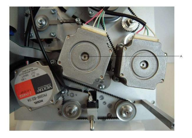
In case the ribbon savings function is activated and you can note that the printhead does not move far away from the label material, it is necessary to adjust the pressure curve anew. This curve is situated onto the axe of the ribbon savings motor (A).
