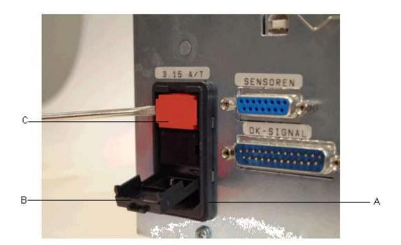
The primary fuse is into the line filter block (A).
