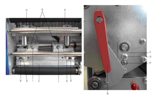
**Note:** Please note that you have to observe the ESD regulations for replacing the printhead! Do not touch the contacts of printhead!
