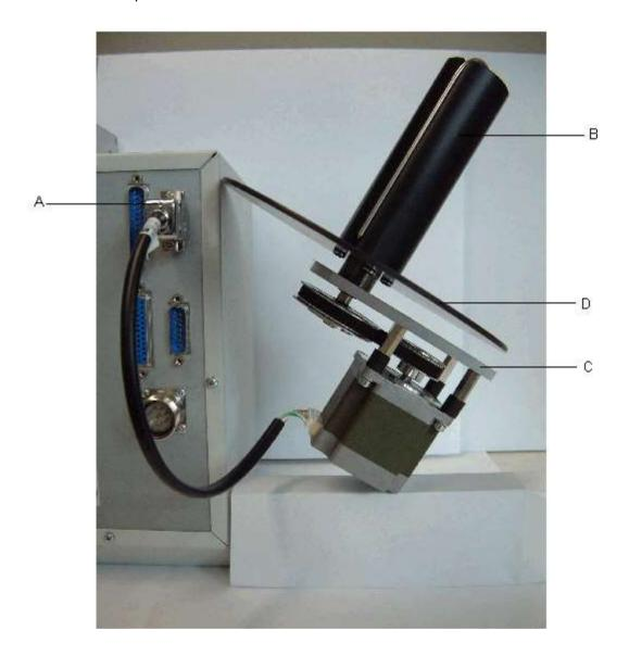
Guide the 9pin DSUB plug (A) of the rewinding unit (B) into the appropriate bushing at the side panel of the print mechanics.
