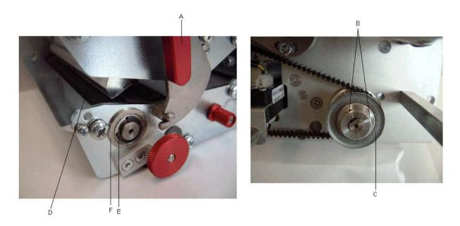
Remove the cover at the rear of the print mechanics Unscrew 2 screws at the rear and 3 at the connection side.
