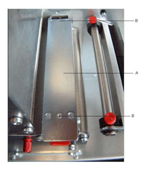
In case at an activated ribbon savings function jamming of paper occur or the position of the print onto the label is not correct, then this could arise because of the wrong setting of rail (A).
