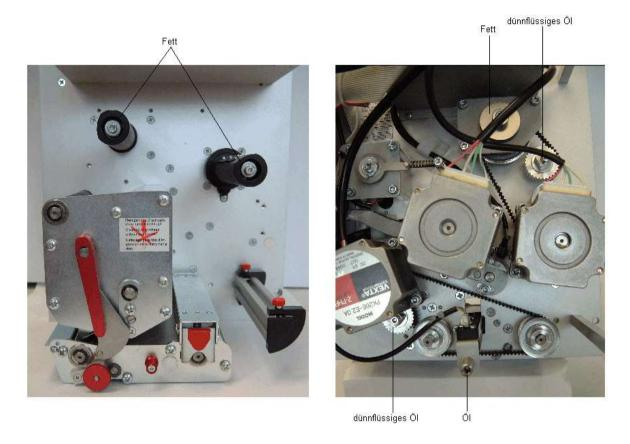
Make sure when oiling and greasing that no lubricants deposit on photocells, electronic components, circuit boards, printhead and rolls.
