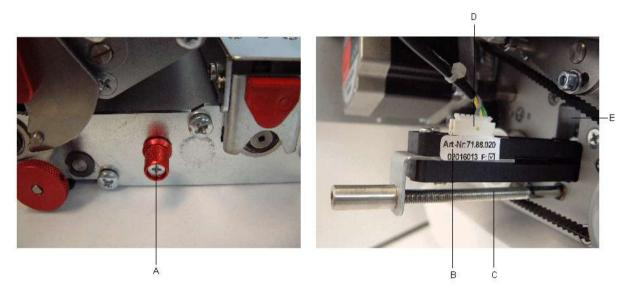
Remove the cover at the rear of the print mechanics Unscrew two screws at the rear and three at the connection side.
